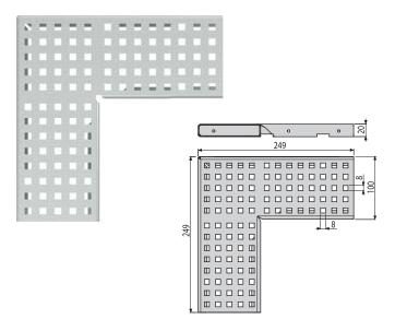
Grid for drainage corner channel 100 mm, stainless steel
